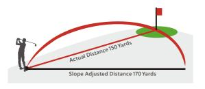
\*When going uphill, the compensation distance will be greater than the straight-line distance. When going downhill, the compensation distance will be smaller than the straight-line distance.
